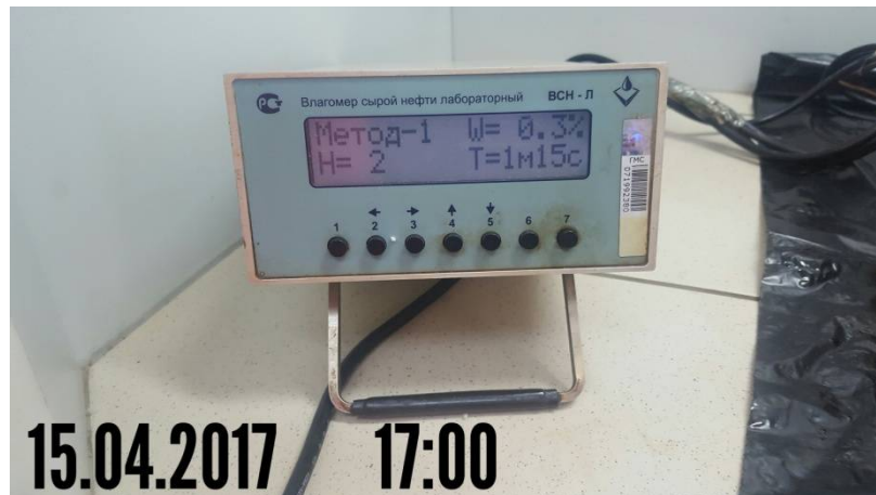
Figure.1. The result of measuring the concentration of residual water after thermochemical treatment of the oil-water emulsion using the nanodemulsifier “IKHLAS” -1 (at a dosage of 90.9 g/t).
