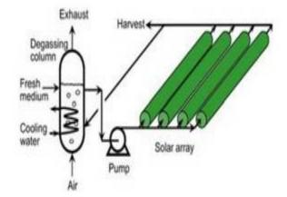
The photosynthesis process generates oxygen. In an open-raceway system, this is not a problem as the oxygen is simply returned to the atmosphere. However, in the closed photobioreactor, the oxygen levels will build up until they inhibit and poison the algae. The culture must periodically be returned to a degassing zone, an area where the algal
