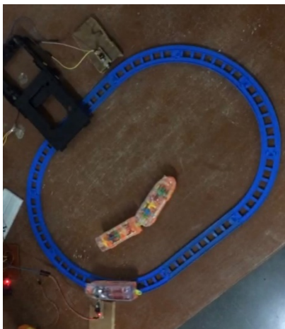
Fig 9 IR sensor senses incoming train
