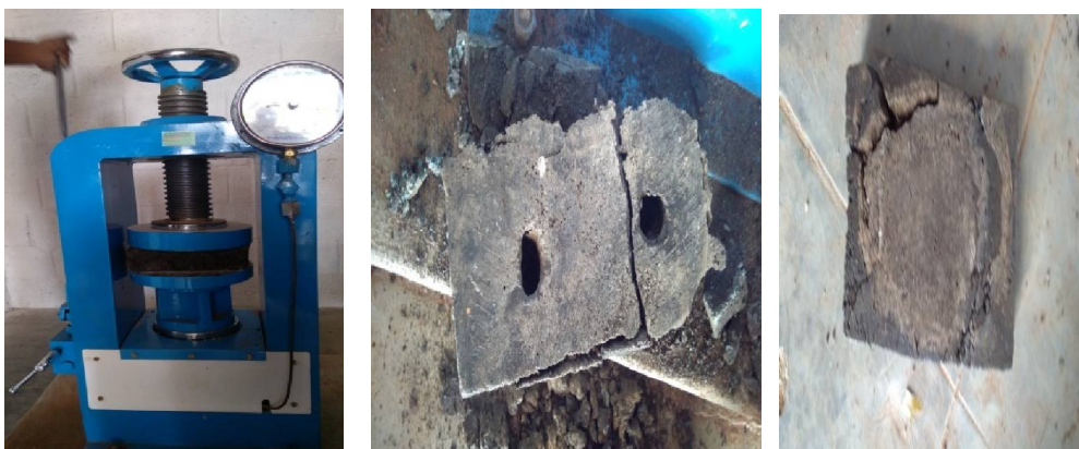
Fig B-1.1 compression strength test on plastic bricks, interlocking bricks & paver block.
