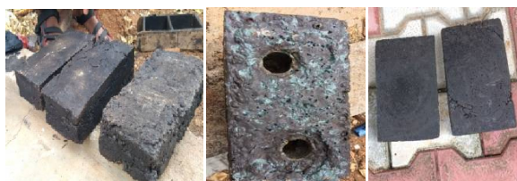
(f) output (Brick, Inter-locking brick & paver block).
