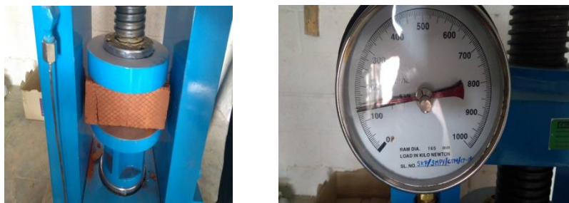
Fig B-1.2 compression strength test on conventional bricks
