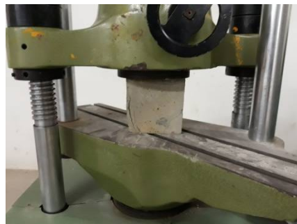
Fig: 3 Compressive strength Test
