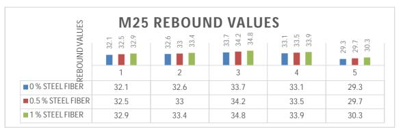
Fig 8: Comparison of M25 Concrete Rebound Values The M25 Grade Rebound test results shows that strength are Good stage
