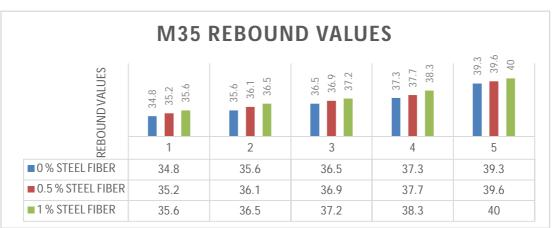
Fig 10: Comparison of M35 Concrete Rebound Values The M35 Grade Rebound test results shows that strength are Good stage
