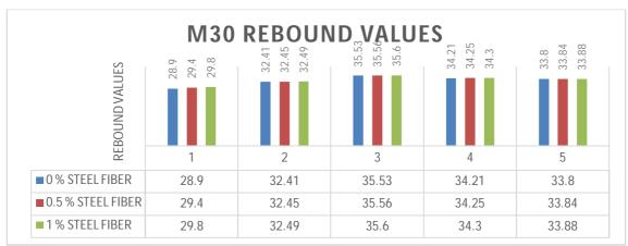
Fig 9: Comparison of M30 Concrete Rebound Values
