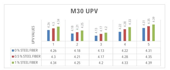
Fig 4: Comparison of M30 Concrete UPV Values in Km/S
