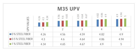
Fig 5: Comparison of M35 Concrete UPV Values in Km/S
