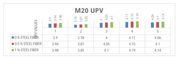
Fig 2: Comparison of M20 Concrete UPV Values in Km/S The M20 Grade UPV test results shows that strength are in the middle of very good to excellent stage
