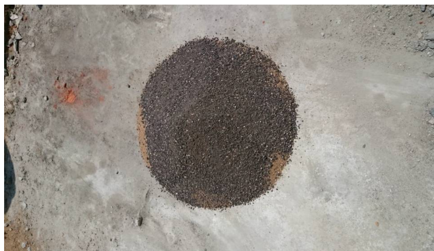
Fig. 2.1 Concrete mix with iron slag
