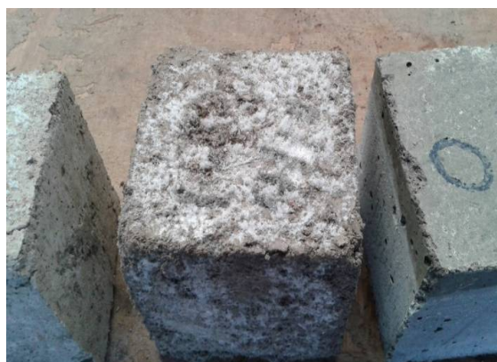
Fig 20: Efflorescence on 100% Cinchona ash Mortar cube.
