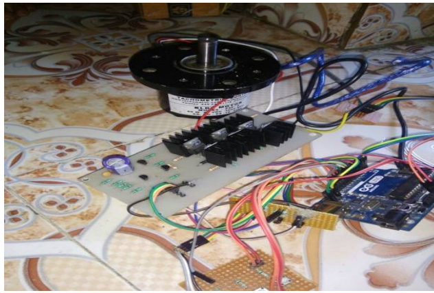
Figure.6 :- hardware connections BLDC motor and inverter with microcontroller.
