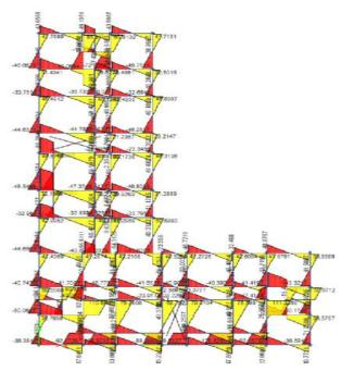
Fig.12 Shear Force Diagram Zone III
