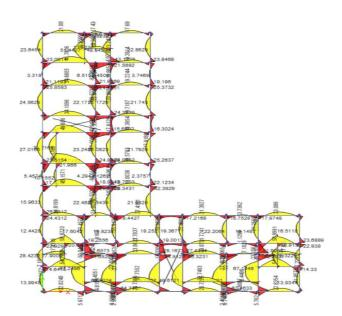
Fig.11 Bending Moment Diagram in Zone III
