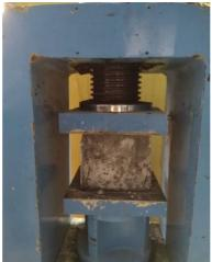
Fig.3. Testing of cube in compression testing machine
