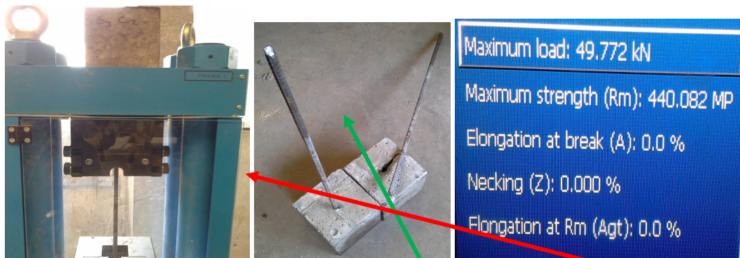
UTM used for bonding test two samples one pulled out and the other breaking
