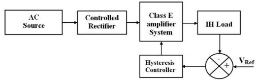
Fig. 2.1 Block diagram of the proposed CEAIHS
