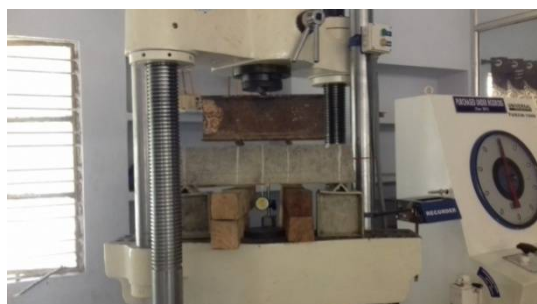
Fig 2 Beam specimen arranged for flexure test on 100T Universal Testing Machine
