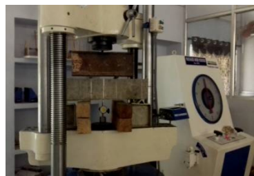
Fig. 3. Details of the test set up with loaded specimen
