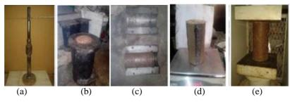
Fig. 1. Sequences involved in preparation and testing of cylinder specimens (a) Tamper used for compaction of cylindrical specimens, (b) Cylindrical mould of 102 mm diameter and 203 mm height used for compaction, (c) Removal of specimen from the mould after 24 hours, (d) Weighing of specimen after proper sealing, (e) Curing of specimens in the BOD incubator at a constant temperature 23.7 °C
