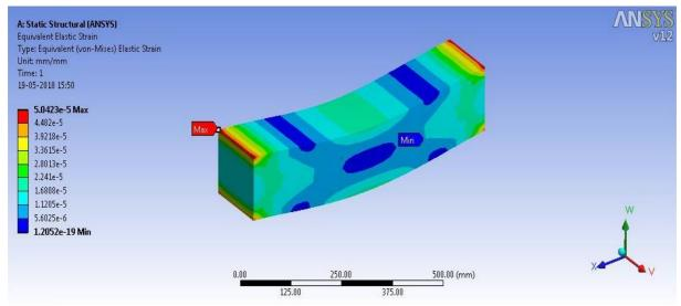
4.2.1 Flexural strength beam conventional concrete equivalent elastic strain value 28 days
