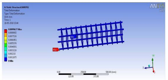
4.1.4 Flexural strength beam equivalent total deformation beam value 14 days
