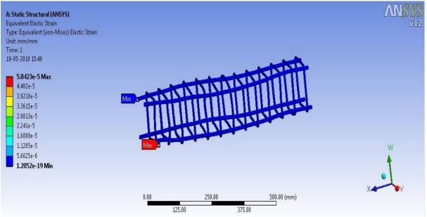
4.2.2 Flexural strength beam conventional concrete equivalent elastic strain value 28 days
