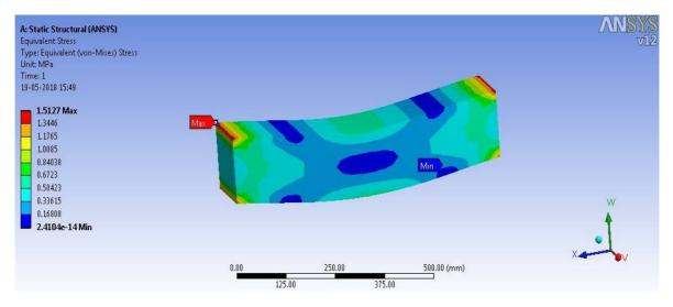
4.2.3 Flexural strength equivalent total deflection beam value 28 days
