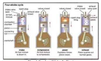
Fig: 4-Strokes Of An Ic Engine
