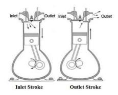
Fig: Compressed Air Engine Working
