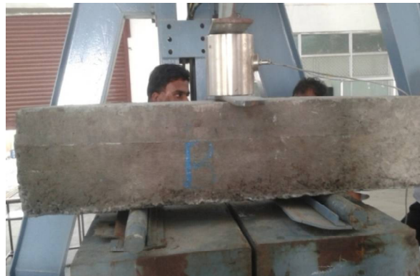
Fig 6 static load test
