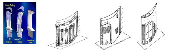
Fig: 2.5(a) Turbine cooling Fig: 2.5(b) Film and Convection cooled Fig: 2.5(c) Impingement cooling Fig: 2.5(d) Transpiration cooling
