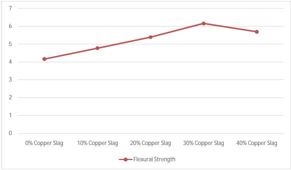
Fig. 3.6: Flexural Strength in MPa
