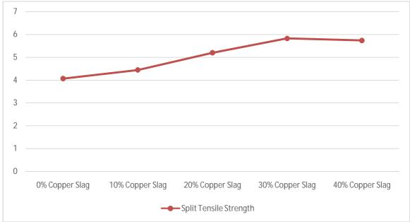
Fig. 3.5: Split Tensile Strength in MPa
