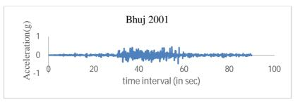
Figure 9: Time Vs Acceleration graph obtained from Bhuj Earthquake data
