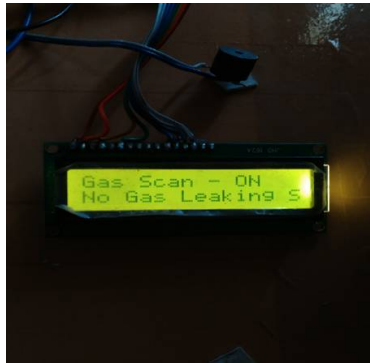
Fig 3 Display of No Gas Leaking
