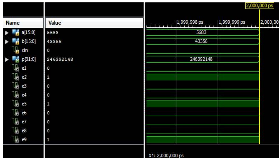
Fig 7: Output waveform of 16-bit multiplier using ripple carry adder
