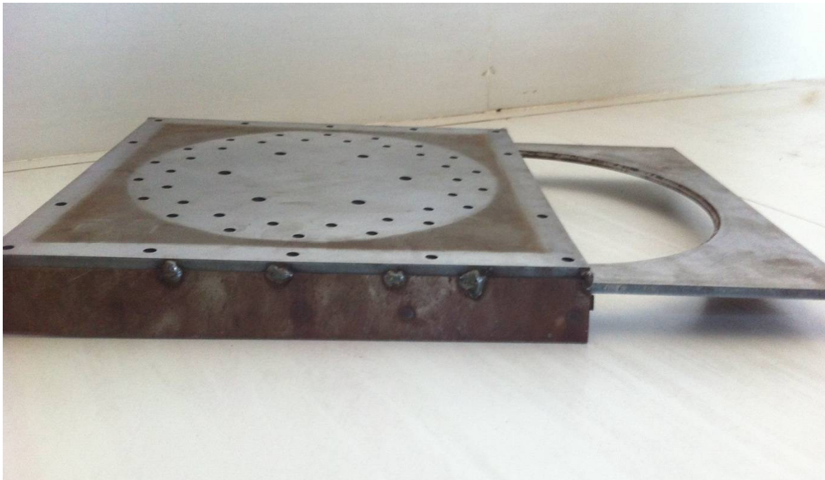
Fig [6] side view of jig with opened sliding tray for holding the work piece
