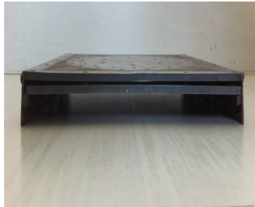
Fig [5] Side view of Sliding tray drill jig
