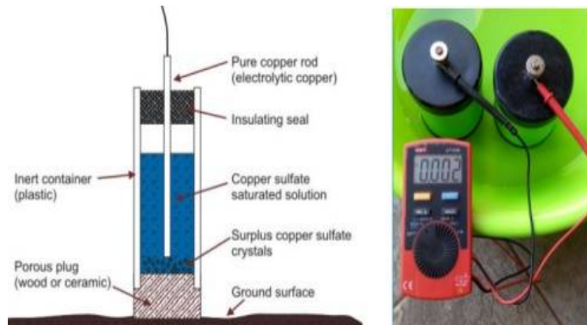
Figure 4. Description of the in-house built non-polarisable electrodes.
