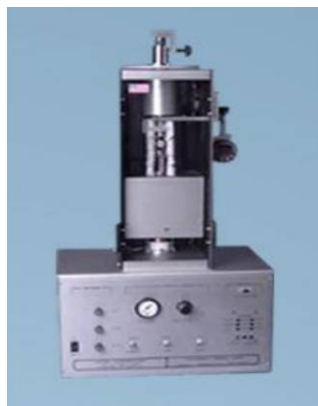
Fig 3 Determination of Thermal Conductivity Using Unitherm™ Model 2022
