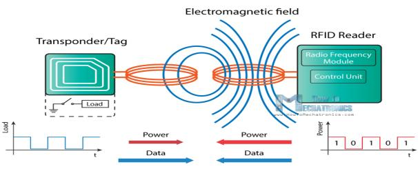
Fig 4:Simple Diagram Showing How RFID Works
