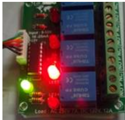
Fig. 8: Turning OFF Load-1 [Fan]
