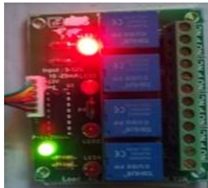
Fig. 7: Turning ON Load-1 [Fan]
