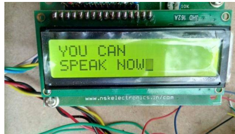
Fig (f): The voice recognition module asserts this message. The victim can speak out loud the key words like "help".
