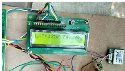
Fig (e): The GPS location of the victim's latitude and longitude will be sent to the Police Station.
