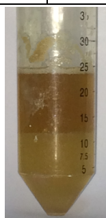
Figure 3: PEG 4000-Ammonium Sulphate ATPS: equilibrated phase volume ratio
