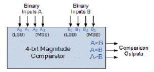
It can compare two 4 bit binary number Aand B and the outcome of comparator has been specified by three binary variables G(A>B), E(A=B), E(A=B).
