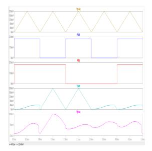
Half subtractor with Fin-FET SAL is designed and simulated by LTspice 45nm technology. For supply voltage 200mv and operating frequency 1 kHz is analyzed.
