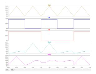
Half adder with Fin-FET SAL is designed and simulated by LTspice 45nm technology. For supply voltage 200mv and operating frequency 1 kHz is analyzed.
