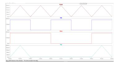
D-Flipflop with Fin-FET SAL is designed and simulated by LTspice 45nm technology. For supply voltage 200mv and operating frequency 1 kHz is analyzed.
