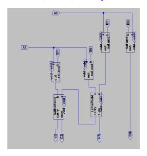
2-bit binary multiplier with Fin-FET SAL is designed by LTspice 45nm technology. For supply voltage 200mv and operating frequency 1 kHz is analyzed.
