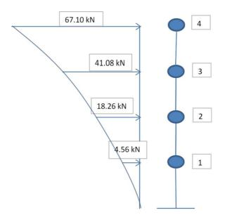
Figure 4.1 Applied Inverted Triangular Loading
