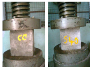
Figure 6.1 Compression test on CC and S40 specimens
