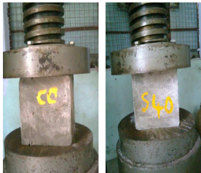
Figure 6.1 Compression test on CC and S40 specimens
