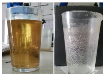
Figure 5. Pronounced crystalline states for a liquid crystal nano-demulsifier of the type LCND formed on the walls of a glass beaker: (1) "IKHLAS" LCND- 6003-20; (2) "IKHLAS" LCND- 5003-15; (3) "IKHLAS"LCND- 4003-12; (4) "IKHLAS" LCND- 3500-10.
