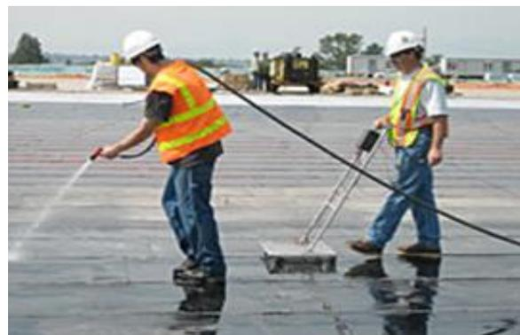
**Figure 4. Low voltage platform in action**
