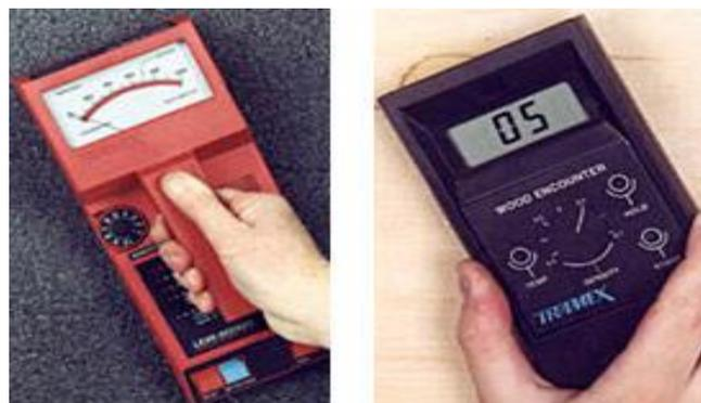
Figure 9. Tramex Capacitance meters
