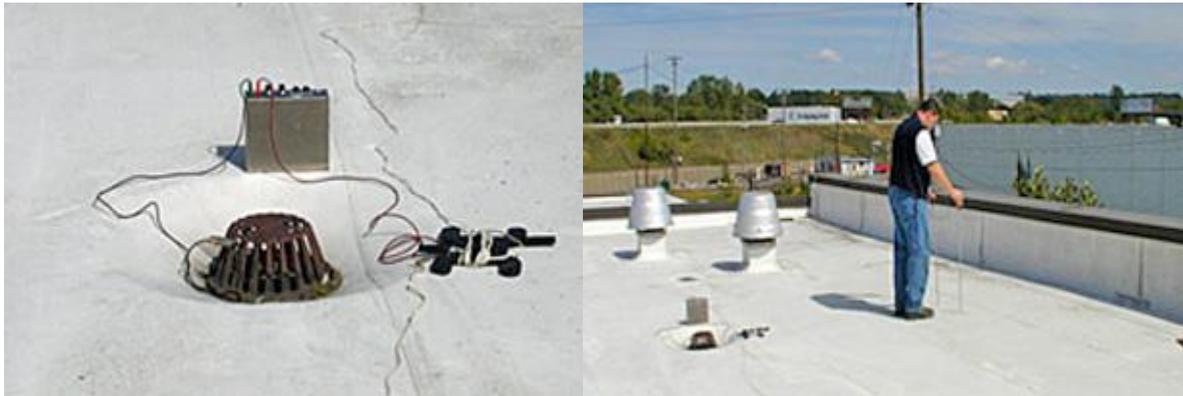
**Figure 2. Low voltage test equipment**
