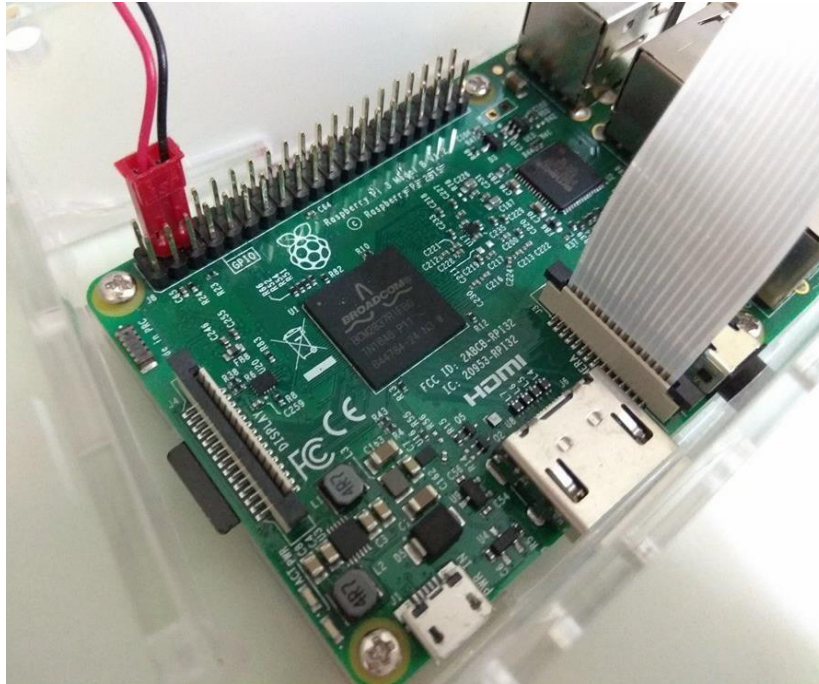
Figure 3.2 Connections of pi-fan and pi-camera onto the raspberry pi 3 board.
