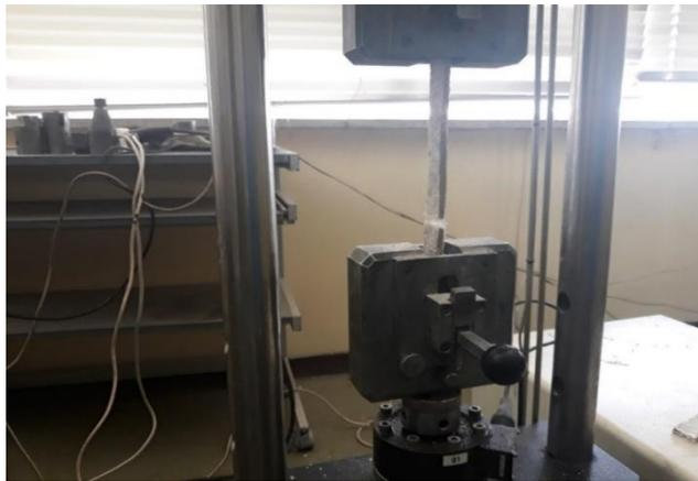
Figure 5. Tensile testing machine
