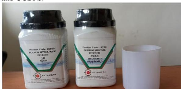
Fig. 2.Some Alkaline Activators
