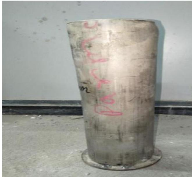
**Fig.4** Behavior of CFST after testing
