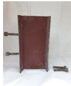
Figure 11 Failure of Headed stud connectors under monotonic loading
