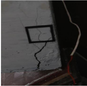
Fig 14. Cracking pattern of Rectangular Rectangular connector specimen failure
