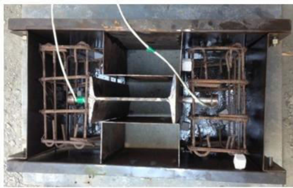
Fig 4. View of concrete casting mould with
