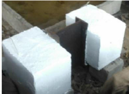
Fig 5. View of composite specimen after curing reinforcement
