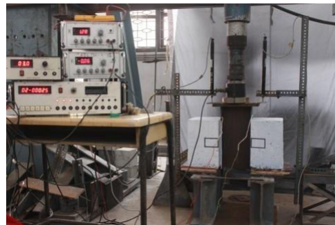
Fig 7. push-out test specimen during testing
