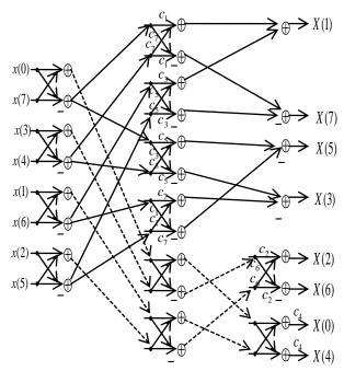
Figure 2: 8-point Discrete Cosine Transform
