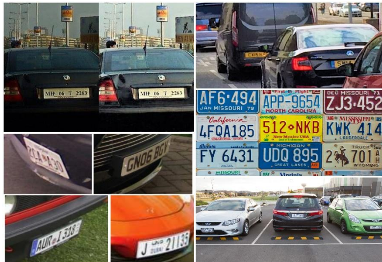
Fig. 2 From top-left (clockwise): Illumination variation; Occlusion; Font variation; Multiple LPs in a frame; Distorted LPs
