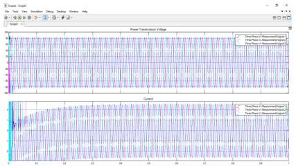
Figure13. Voltage and Current of DC-AC Converter
