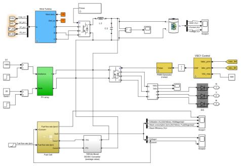
Figure2. PV/WT and FC to DC-DC bus and DC-AC Bus
