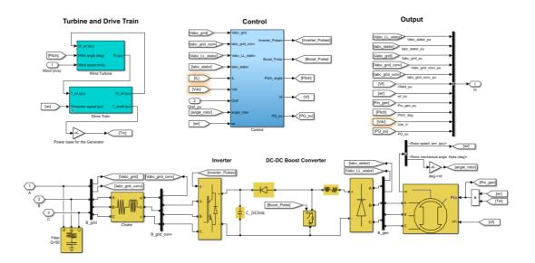
Figure4. Modelling of WT with converters
