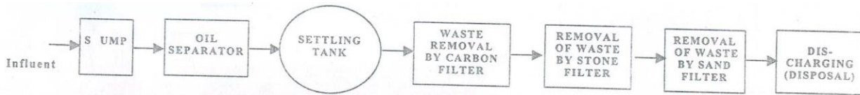
Fig. 2 Treatment process in Kodai automobiles service station.
