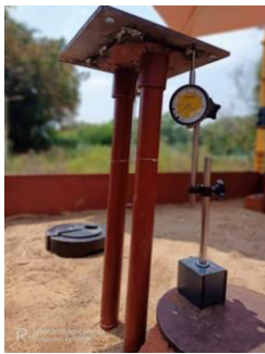
Fig 5: Arrangement of Pile group with 2-piles
