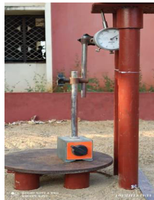
Fig 2 : Setup of pile with dial gauge
