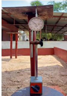
Fig 3: Loading set up on a single pile
