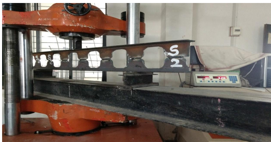
Fig. 3 Testing of IS2 castellated beam under UTM
