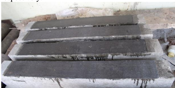
Fig 6: Beams with Flexural Strengthening
