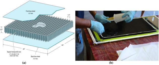
Figure (a)Sandwich Structure panel, (b)Preparation of face sheets
