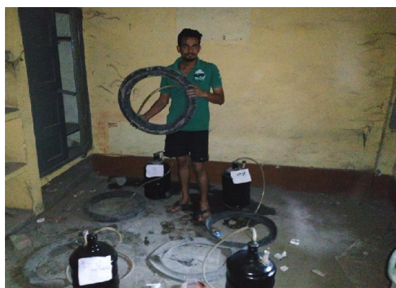
Figure 3. Digesters with different waste (PHASE 2)
